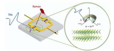
2D TMD embedded in a THz split ring cavity (left) The resulting coupled light-SC matter state is probed by Raman and THz spectroscopy. The SC Higgs mode is a collective oscillation of the SC condensate (right) that can couple to cavity photon to form cavity-Higgs polariton
